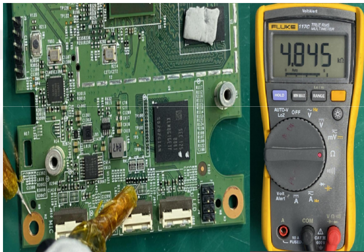
Measure impedance at R2954 location
