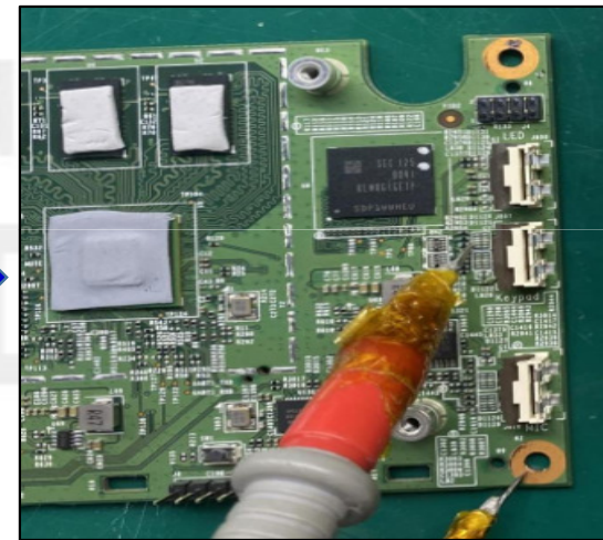
Check power at R2954 location when connect internet
